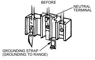
C. Insert screws through each power cord terminal ring and into connector block until screw engages nut. Be certain that the center wire is connected to the center screw of the connector block. Tighten screws securely.
